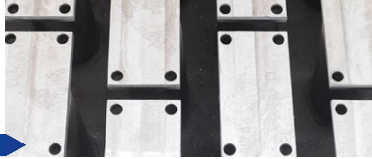
Surface cleaning and overlay welding followed by face milling
