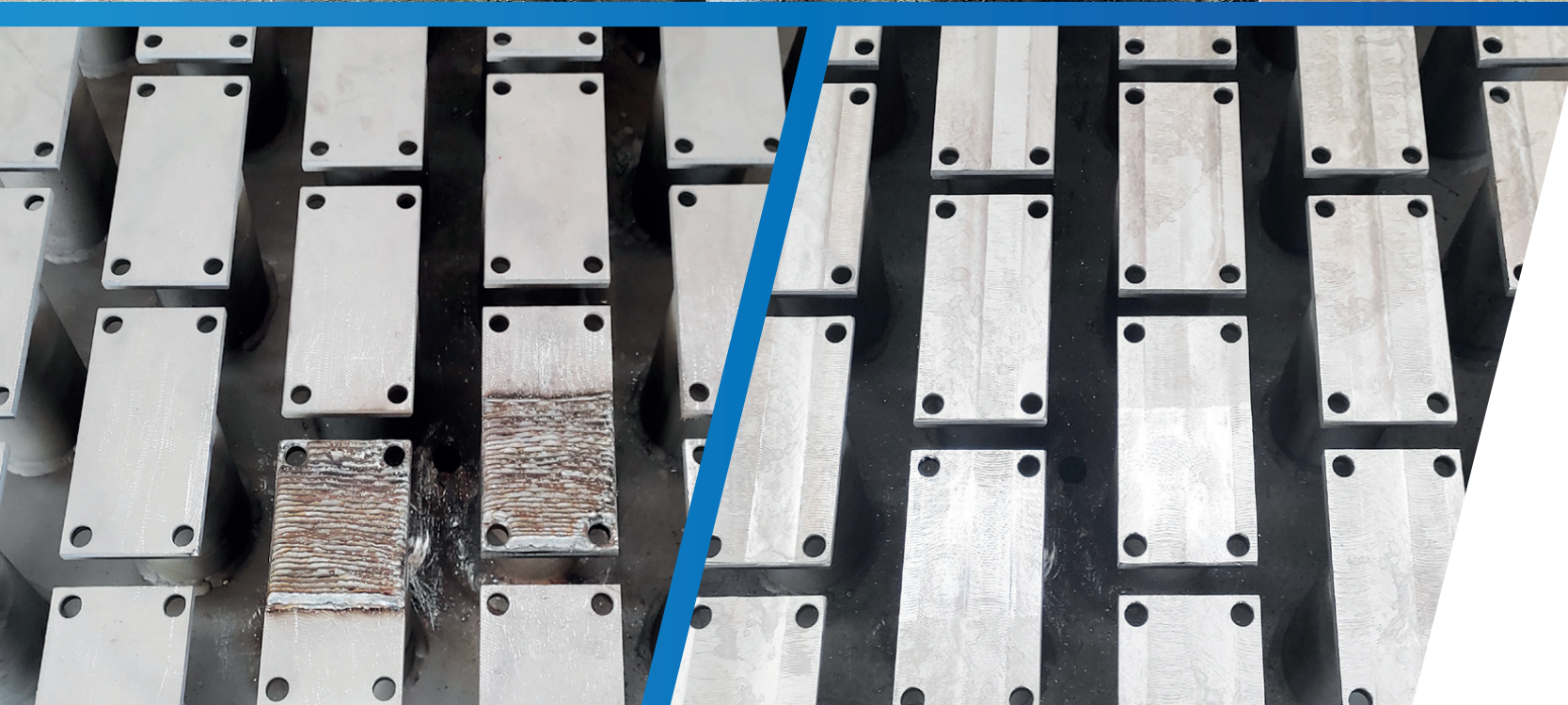
Surface cleaning and overlay welding followed by face milling
